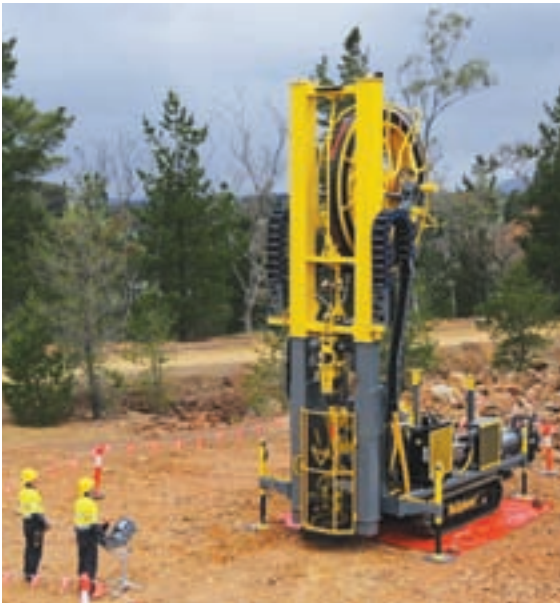
The RoXplorer CT drilling rig ► DET CRC says that coiled-tubing (CT) drilling can provide the step reduction in drilling costs required to increase the success of mineral exploration beneath barren cover.
