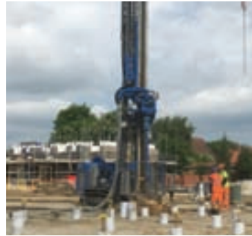
The new Comacchio MC 13 F drill rig, equipped with safety guard and devices in conformity with the European safety standard EN16228
