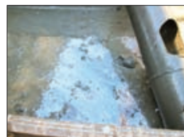
Drill spoils and water contaminated with old bunker oil
