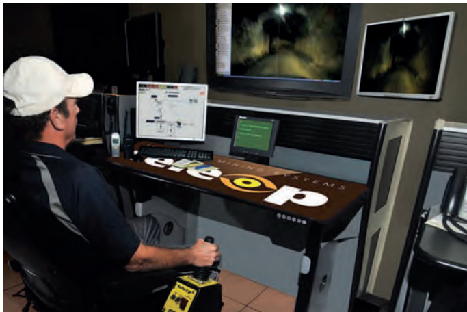
Teleop AutoX will allow for an operator to run multiple machines automatically that can be programmed for multiple destinations
