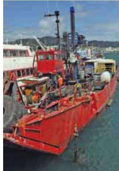
The Brandywine craft with Sonic Drill installation on board, used for iron sands exploration in 2011
