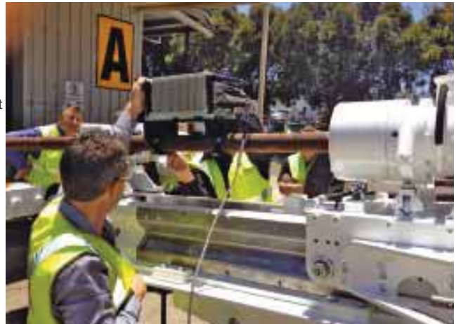
The DHS Azimuth Aligner installed on a Swick drill rig
