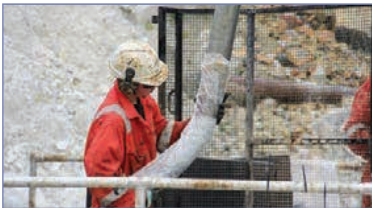
Sonic drilling allows the recovery of 100% intact core samples
