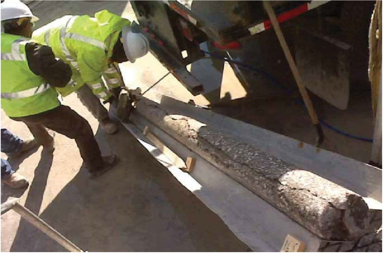
Figure 4. Sonic core of cut-off wall panel seam.
