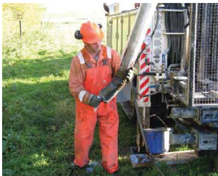
Figure 2. Extrusion of sonic core into plastic sleeve.
