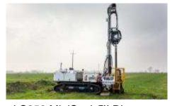
LS250 MiniSonic<sup>™</sup> Rig: Compact footprint rig with a proven sonic head that delivers continuous 'in-situ' core samples.
