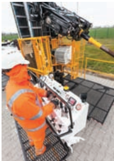
Boart Longyear’s LF160 surface coring rig with optional rod handler
