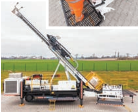
Boart Longyear’s LF160 surface coring rig with optional rod handler
