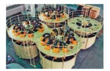
for perfect separation is constant pressure at the hydrocyclone inlet. The system is designed to enable pressure variations to be counterbalanced by a speed-controlled pump.
