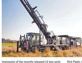
rig. With advanced sonic drill technology featuring innovative and patented designs, the LS600 delivers continuous-undisturbed core samples and will be onsite at MINExpo.
