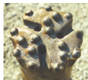
(left): Harder ground conditions and drilling with excessive rotation creates wear that tends to be greater on the bit circumference; (right): Body wash often occurs when drilling in non-abrasive materials
