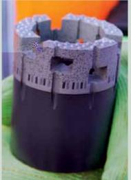
The arrangement of these protrusions also improves tracking and balance in the hole when drilling begins.
