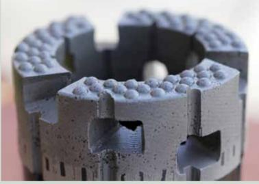
In addition, the bits did not require extreme measures to remain sharp, and the drillers were able to maintain the proper torque on the rigs while sustaining a continuously sharp bit.
