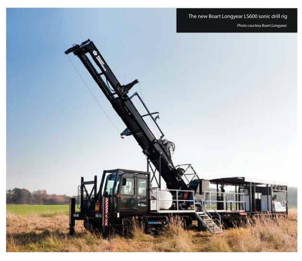
The vibrating sonic drill head is designed to produce frequencies of up to 150 Hertz, which matches the resonant energy of the ground, allowing the core barrel to easily advance through unconsolidated and difficult overburden formations. Of note, during drilling operations, the borehole is continuously cased by first allowing the core barrel to advance into the substrate, followed by the outer casing.
